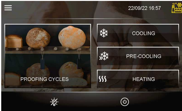
Retarding-proofing Home screen (E12=1)
