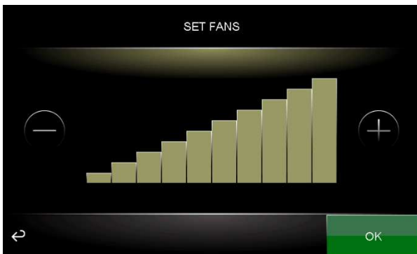
Selecting fan speed (e.g. with 10 speeds)
